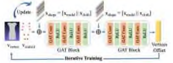
Figure 4: Details of the GAT based deformation module. The input contains clothing meshes and control points, as well as clothing and model features extracted by CNN extractors. The output is the vertex’s coordinate offset. An iterative training strategy is adopted to optimize the result. For each iteration, model features will be recalculated according to the updated vertices coordinates.
